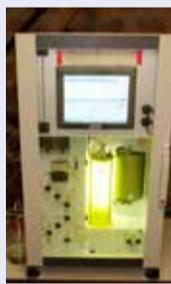
The fluorescence of algae in a Rhinewater sample is compared in 30-minute intervals with a control sample of algae in drinking water. Any significant difference
